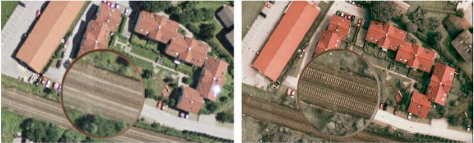
Figure 6: Color image segment from aerial film (left) with a GSD of 15 cm, obtained from a 12.5\mu\text{m} scan. The UltraCam-image has a GSD of 16 cm (right). The inserts are 2x enlarged and have a diameter of 150 pixels. Note the definition of the railroad track.
