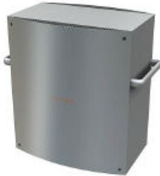
Figure 7: The UltraCam-D/SCU storage and computing unit for distributed parallel UltraCam data collection and on board processing. A total of 15 CPUs and 30 (mobile) hard disks collect and process up to 1 Tbyte of data at a minimum interval of 0.75 seconds per image take. For dimensions and weight see Table 1.
