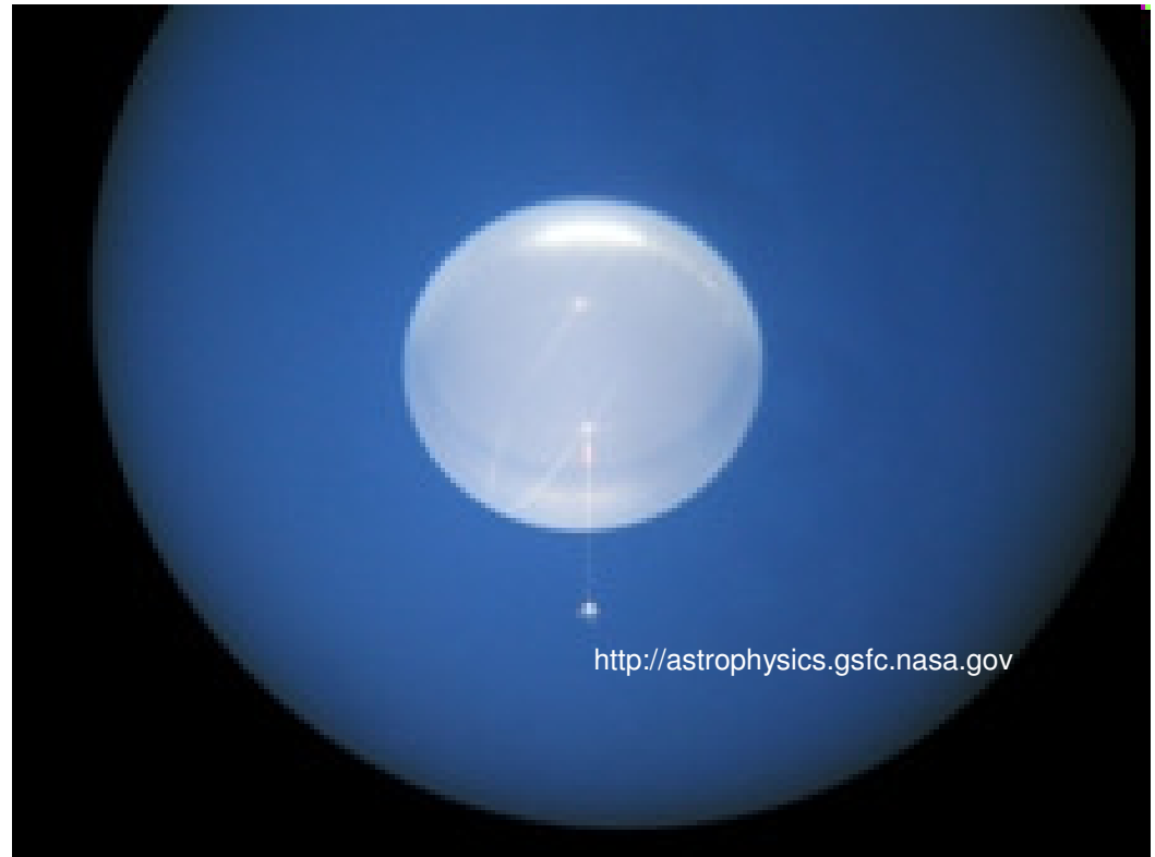
This image, taken through a telescope, is of the newly designed super pressure balloon at float altitude over Antarctica.
