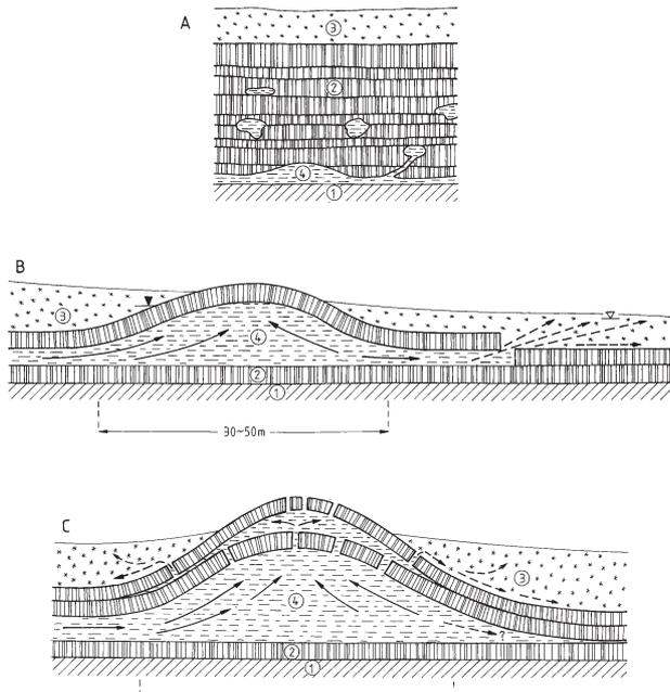
**Fig. 2.** Naled drainage schemes
