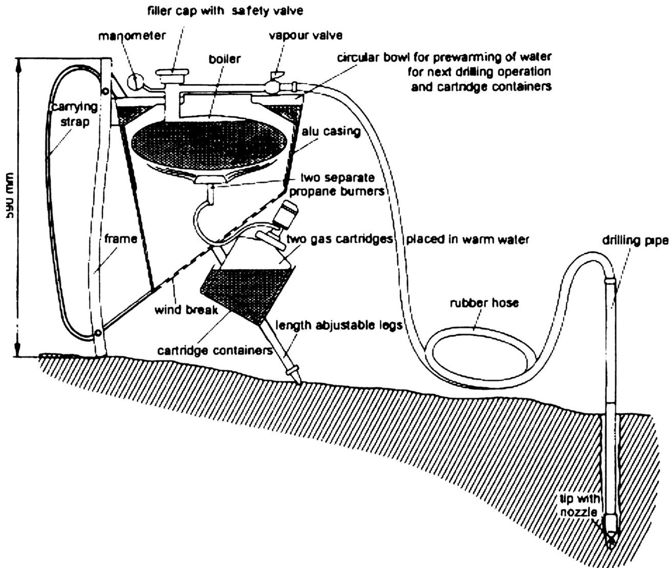
Fig. 2. Diagram of the entire drilling device
