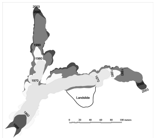
Fig. 4. Development of the Puriceni gully system within Falcu Hills over the period 1956–2003 using aerial photos and topographic leveling
