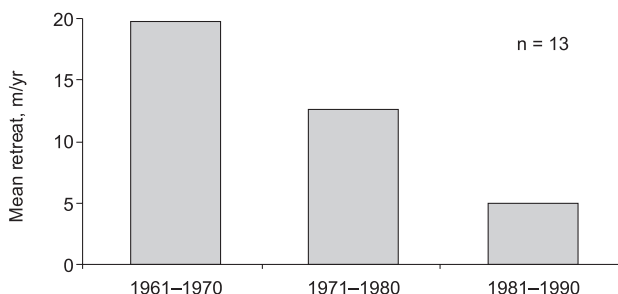
Fig. 2. Measured gully head retreat in the Moldavian Plateau between 1961–1990
