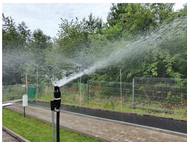
Fig. 5. Nozzle used for rainfall simulation
