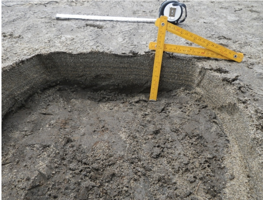
Figure 7. Tsunami deposit at site 3-30 (1.45 km from shore, Natori City) composed of 7 cm thick sand overlain by 5 mm thick mud.
