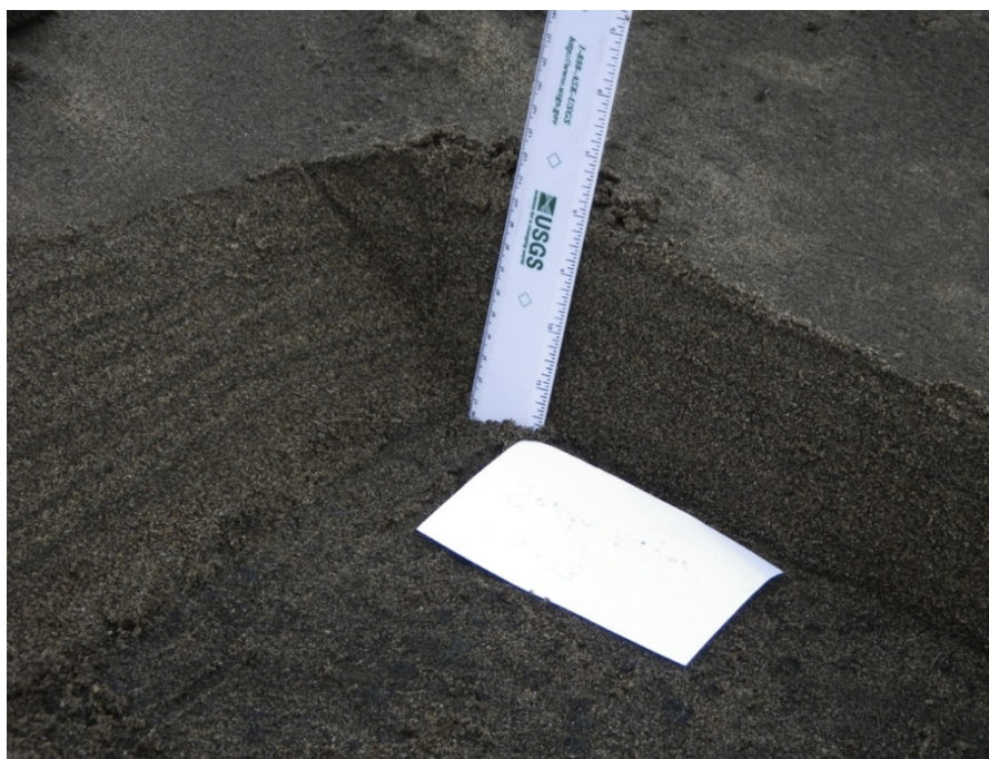
Figure 6. 20 cm thick tsunami sand deposit at site 3-12 (550 m from shore, Natori City).
