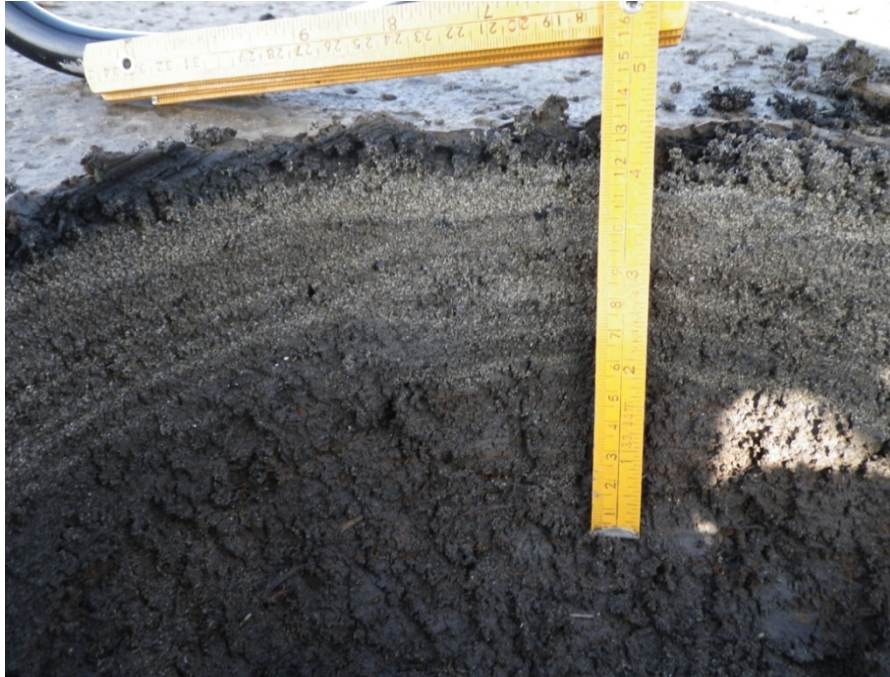
Figure 12. Tsunami deposit at site 3-48 (2.35 km from shore, Natori City) showing a 7 cm thick sand covered by 1.0-1.5 cm thick black mud.
