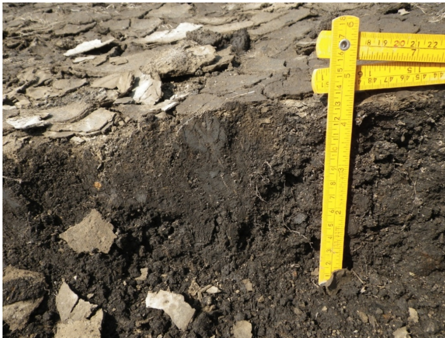
Figure 8. Tsunami deposit at site 3-64 (3.15 km from shore, Natori City) represented by a 5 mm thick mud layer.
