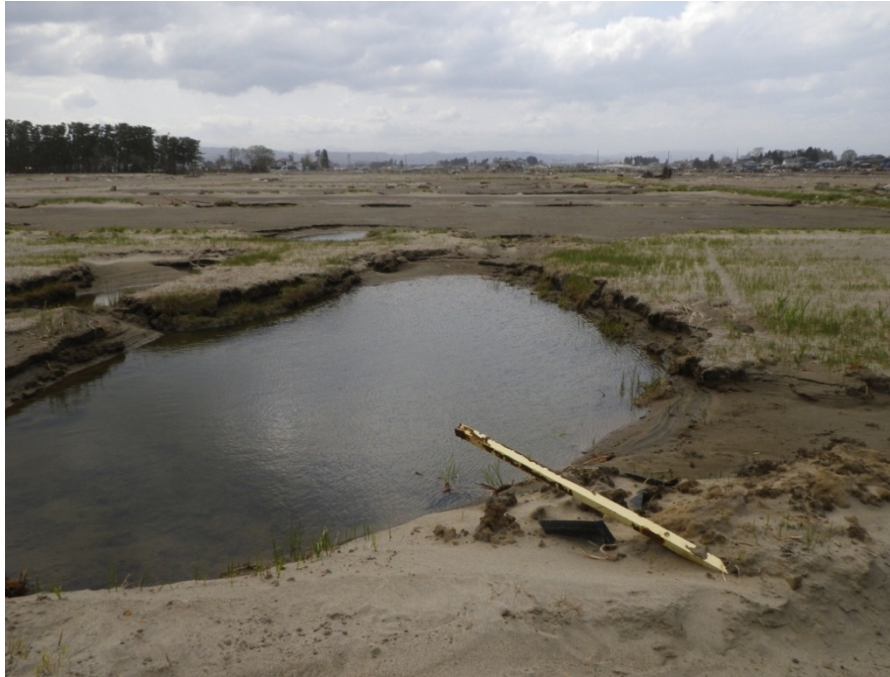
Figure 10. Possible liquefaction features close to site 3-32 (1.55 km from shore, Natori City). The depressions are thought to be due to sand liquefaction and collapse of the surface soil and were likely modified by erosion by tsunami waves. Liquefied sands would have been entrained and transported inland by the tsunami.
