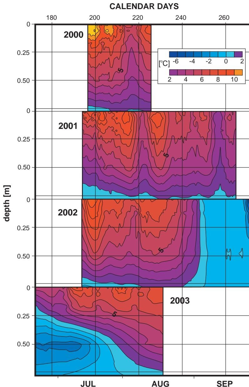
Fig. 8. Temporal changes of ground temperature with depth below ground surface for the summer seasons 2000–2003.
