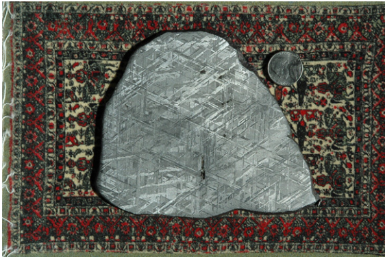
Fig. 1. Polished iron meteorite with Widmanstätten structures. From Korotev (2007).
