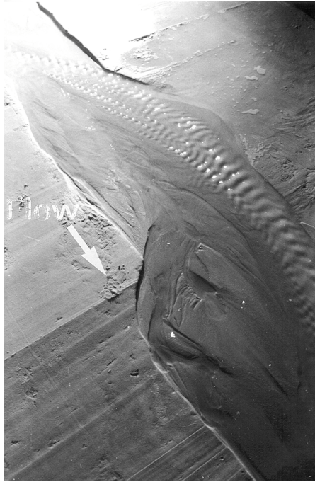
Figure 9.3 View of a train of standing waves along the thalweg of the main 'active' channel in a 1:20 braided gravel-bed river FSM study (Ashworth et al. 1992b). Flow is from top to bottom and the braidplain is approximately 1 m wide. Avulsion of the main channel has left an abandoned channel complex along the right bank and flow is concentrated into one dominant channel which is eroding the outer left bank at the beginning of full braidplain development
